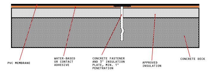
APPROVED INSULATION: UL CLASSIFIED POLYISOCYANURATE INSULATION.
