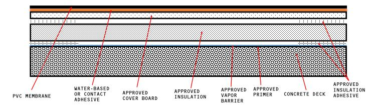
APPROVED COVER BOARD: DENS DECK, DENS DECK PRIME OR SECUROCK GLASS-MAT, MINIMUM 1/4" THICKNESS.
