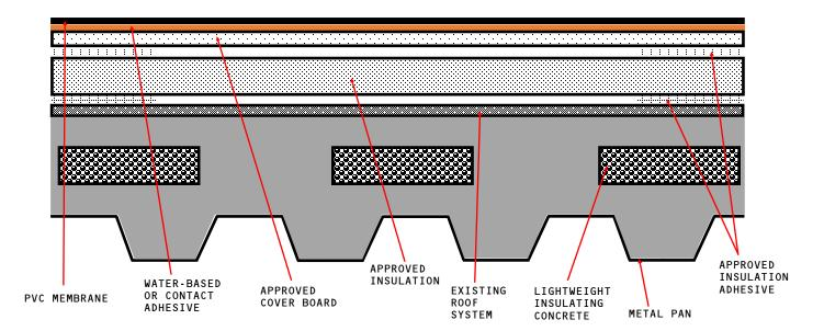
APPROVED COVER BOARD: DENS DECK, DENS DECK PRIME OR SECUROCK GLASS-MAT, MINIMUM 1/4" THICKNESS. APPROVED INSULATION: UL CLASSIFIED POLYISOCYANURATE, EXPANDED POLYSTYRENE, EXTRUDED POLYSTYRENE INSULATION.
