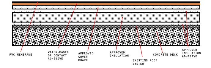
APPROVED COVER BOARD: DENS DECK, DENS DECK PRIME OR SECUROCK GLASS-MAT, MINIMUM 1/4" THICKNESS. APPROVED INSULATION: UL CLASSIFIED POLYISOCYANURATE, EXPANDED POLYSTYRENE, EXTRUDED POLYSTYRENE INSULATION.
