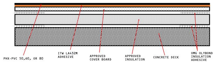
APPROVED COVER BOARD: DENS DECK, DENS DECK PRIME OR SECUROCK GLASS-MAT, MINIMUM 1/4" THICKNESS. APPROVED INSULATION: HUNTER PANELS, RMAX OR ATLAS UL CLASSIFIED INSULATION.
