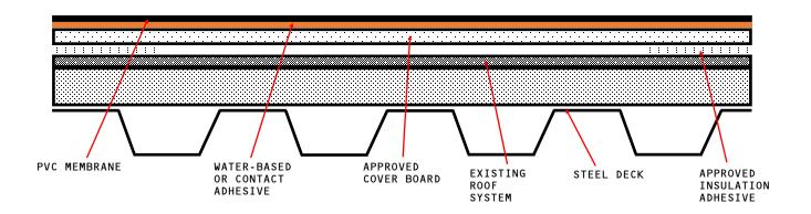
APPROVED COVER BOARD: DENS DECK, DENS DECK PRIME OR SECUROCK GLASS-MAT, MINIMUM 1/4" THICKNESS.
