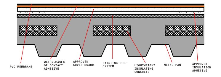
APPROVED COVER BOARD: DENS DECK, DENS DECK PRIME OR SECUROCK GLASS-MAT, MINIMUM 1/4" THICKNESS.
