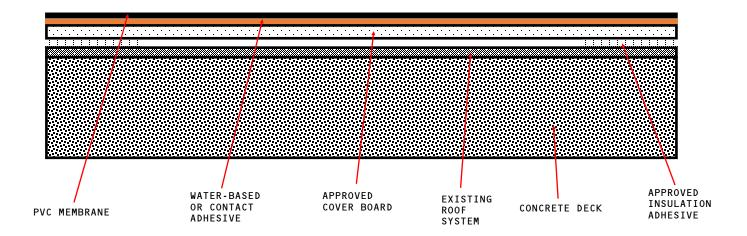
APPROVED COVER BOARD: DENS DECK, DENS DECK PRIME OR SECUROCK GLASS-MAT, MINIMUM 1/4" THICKNESS.
