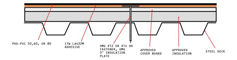
APPROVED COVER BOARD: DENS DECK OR DENS DECK PRIME, MINIMUM 1/4" THICKNESS. APPROVED INSULATION: HUNTER PANELS, RMAX OR ATLAS UL CLASSIFIED INSULATION.
