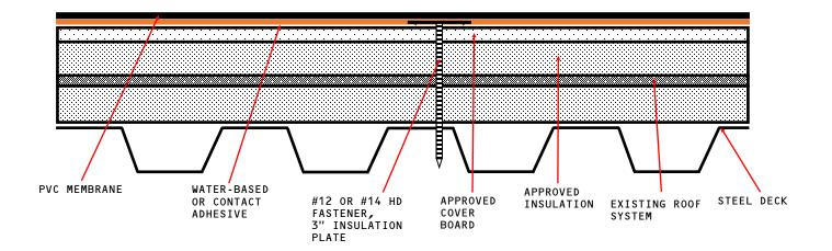
APPROVED COVER BOARD: DENS DECK, DENS DECK PRIME OR SECUROCK GLASS-MAT, MINIMUM 1/4" THICKNESS. APPROVED INSULATION: UL CLASSIFIED POLYISOCYANURATE, EXPANDED POLYSTYRENE, EXTRUDED POLYSTYRENE INSULATION.
