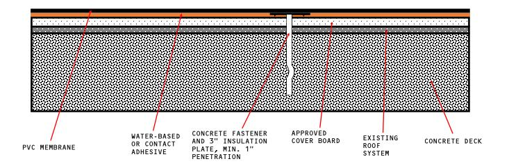
APPROVED COVER BOARD: DENS DECK, DENS DECK PRIME OR SECUROCK GLASS-MAT, MINIMUM 1/4" THICKNESS.
