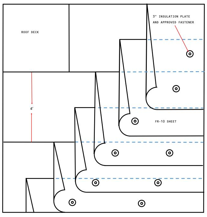
NOTE: SPOT ATTACH FR-10 STAGGERED AS NECESSARY
