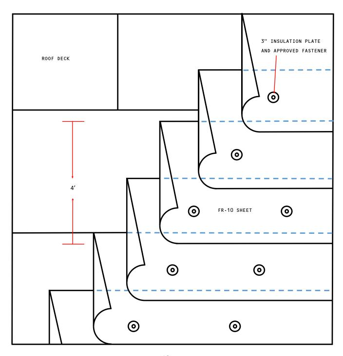
NOTE: SPOT ATTACH FR-10 STAGGERED AS NECESSARY
