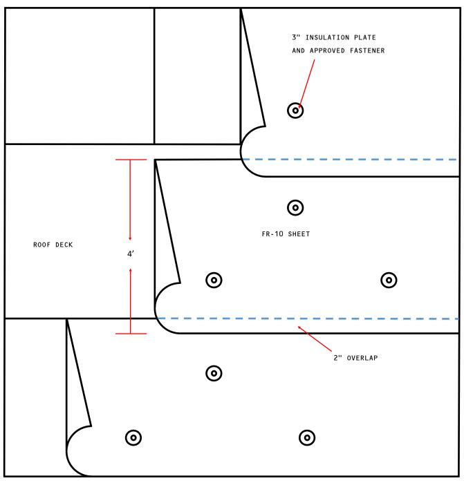
NOTE: SPOT ATTACH FR-10 STAGGERED AS NECESSARY
