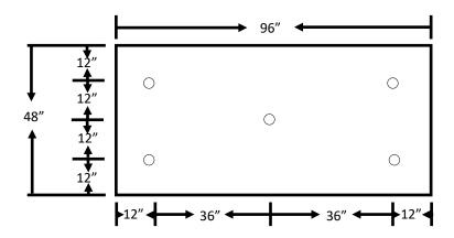
APPROVED RIGID EPS, XPS, POLYISOCYANURATE INSULATION, AND COVERBOARD PHX APPROVED FASTENERS, 3" INSULATION PLATE 5 PER 4'X8'
