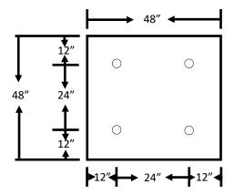
APPROVED RIGID EPS, XPS, POLYISOCYANURATE INSULATION, AND COVERBOARD PHX APPROVED FASTENERS, 3" INSULATION PLATE 4 PER 4'X4'
