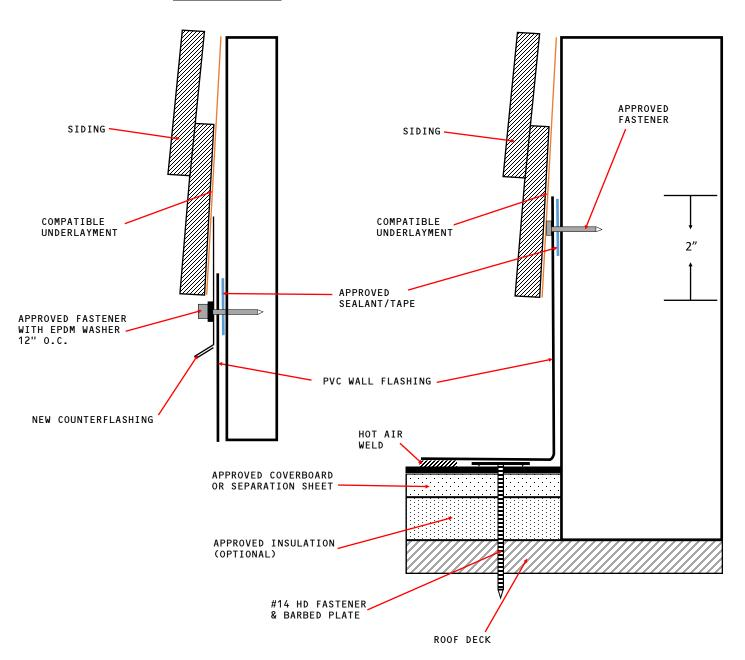
NOTES: REFER TO MECHANICALLY FASTENED OR GLUE DOWN TALL WALL DETAILS FOR ELEVATIONS OVER 18"
